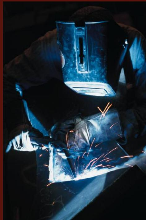
And, cooking is the Welding Process- Passes, Process, Filler Metal, Current, Volts, Travel Speed and Joint Details. Like baking a
